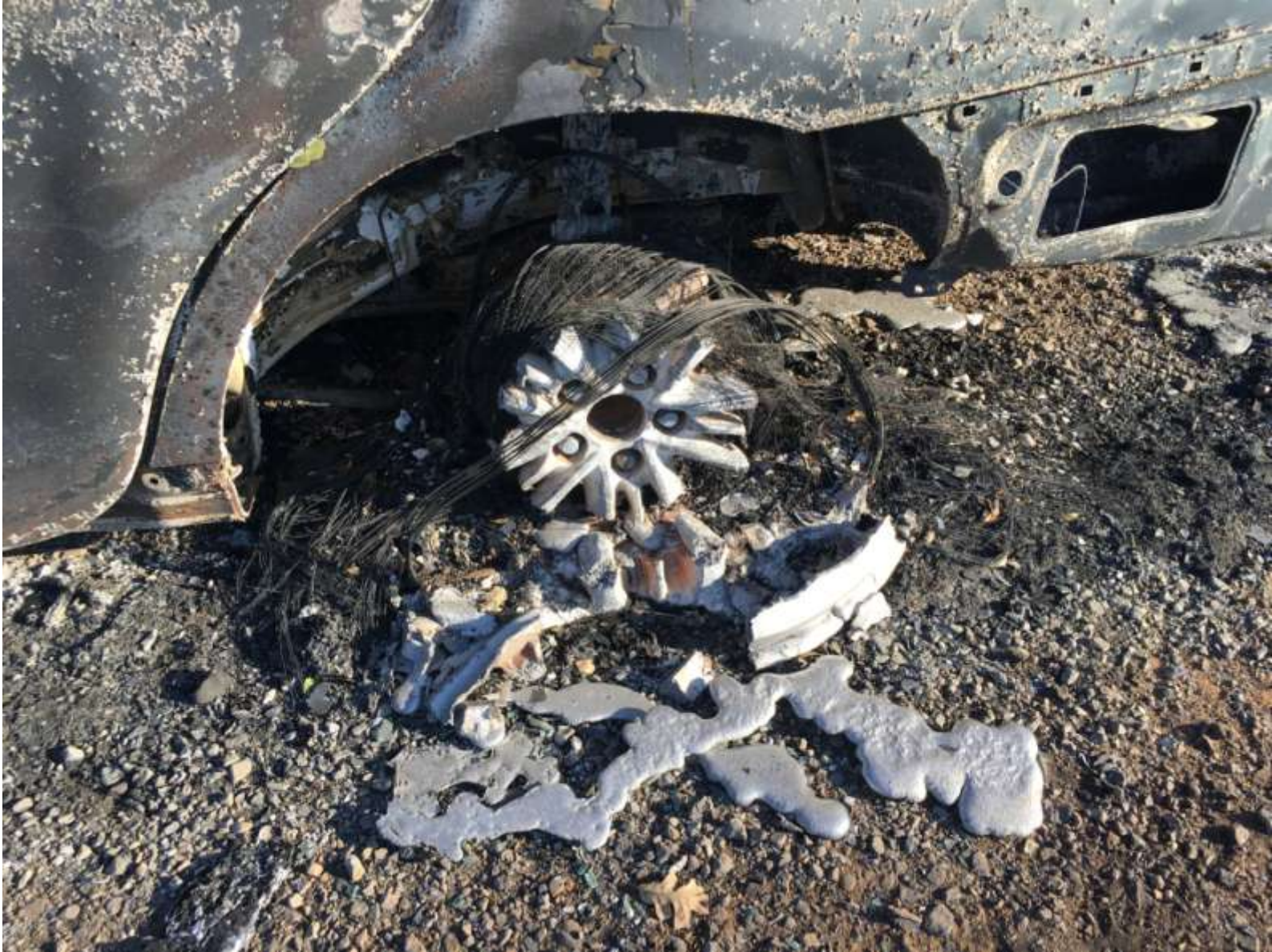
Portrait of a steel-belted radial tire after a fire: The molten metal at bottom is the tin or aluminum or whatever of hubcap, while the wires in middle are the steel belts – the rubber tire completely burned away
